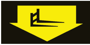
Fork lift point
